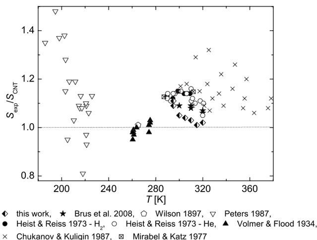
FIG. 7. Temperature dependence of the experimental saturation ratio to critical saturation ratio calculated by CNT.
