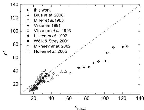
FIG. 9. Critical cluster sizes, determined from the slopes of experimental nucleation isotherms, compared to theoretical prediction by Kelvin equation.
