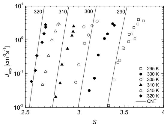
FIG. 5. The isothermal experimental nucleation rates of water,  $J_{\text{exp}}$ , as a function of its saturation ratio,  $S$ , in a comparison to CNT prediction.
