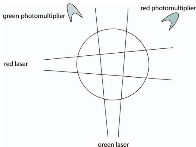
FIG. 4. Schematic figure of coincident counting.
