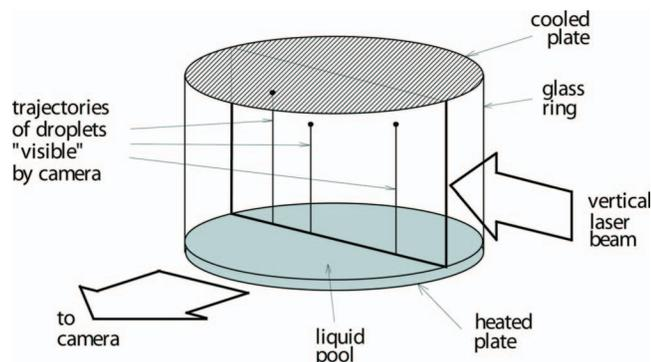
FIG. 2. Schematic figure of the photographic method.
