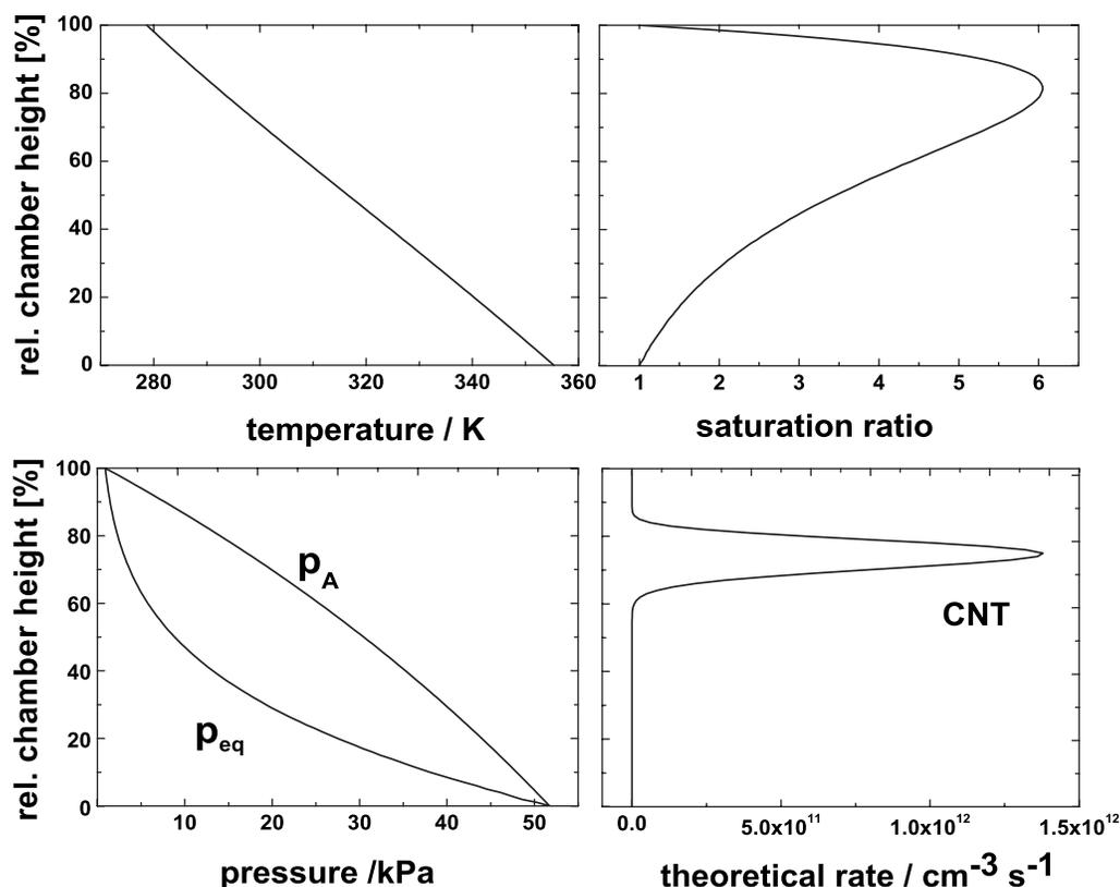
FIG. 1. Vertical profiles of temperature, partial and equilibrium vapor pressure of water, saturation ratio, and nucleation rate inside the TDCC.
